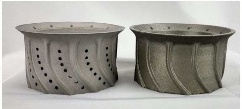
Parts shown for comparison purposes: (L) Unijet™ 17-4PH 75um Binder Jetting - (R) UniFuse™ Ti64 60um LPBF
